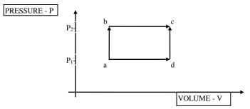
**9**. The figure shows a thermodynamic cycle adcda which a gas may be taken starting at a. Temperatures are: At a T=300K; at b and d T=600K and at c T=1200K. At a the pressure is 100kPa and the volume of the gas is  $1.0m^{3}$ .
